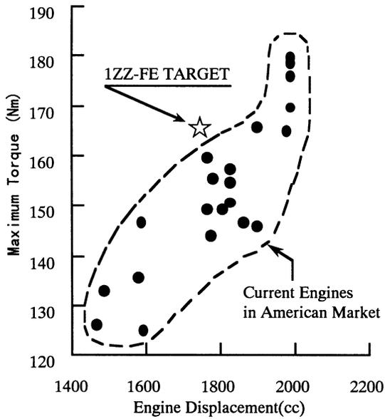
Figure 2. Maximum Torque Comparison
