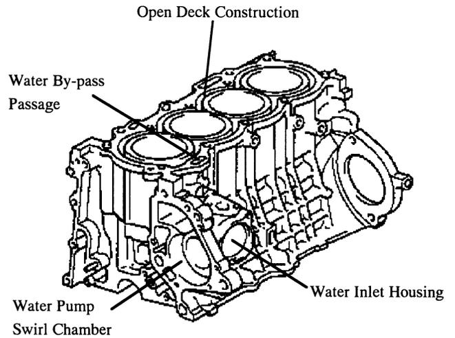
Figure 18. Cylinder Block
