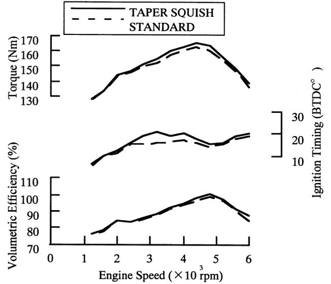
Figure 14. Effect of Taper Squish Combustion Chamber
