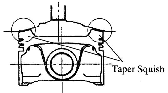
Figure 10. Taper Squish Combustion Chamber
