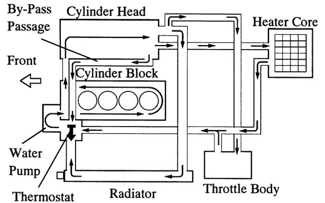
Figure 15. Cooling System
