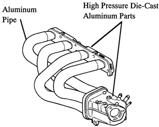
Figure 16. Intake Manifold
