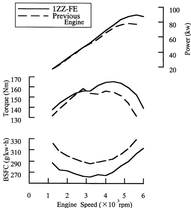
Figure 6. Engine Performance Curves
