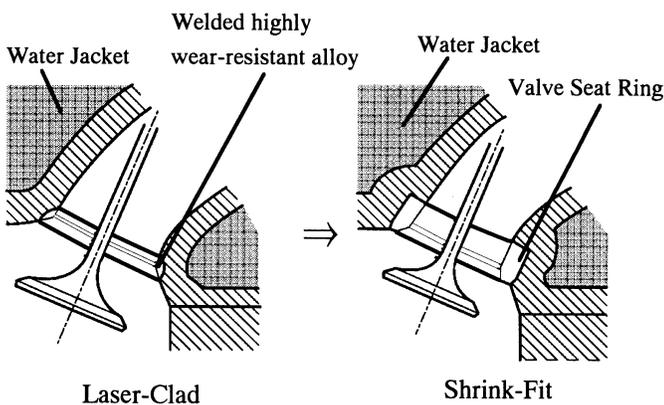
Figure 8. Adoption of Laser-Clad Valve Seat
