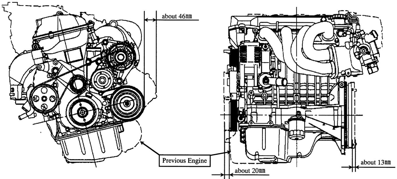
Figure 5. 1ZZ-FE Appearance and Comparison of Dimension
