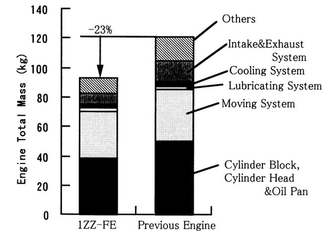
Figure 17. Engine Mass Comparison
