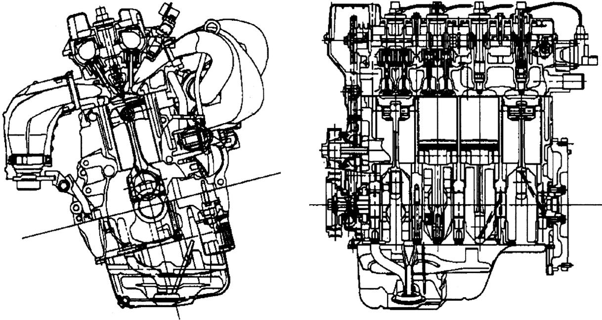
Figure 4. 1ZZ-FE Engine Cross-Sections
