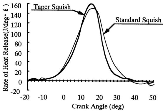
Figure 12. Comparison of Combustion Pattern
