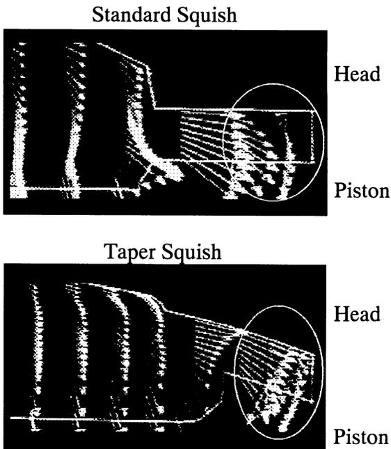
Figure 13. Comparison of Flow Velocity at Squish Area (CFD Simulation)
