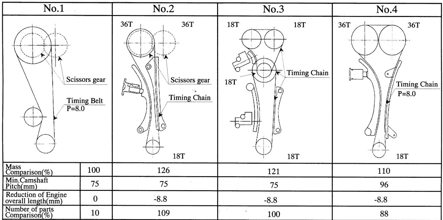
Figure 19. Comparison of Camshaft Drive System
