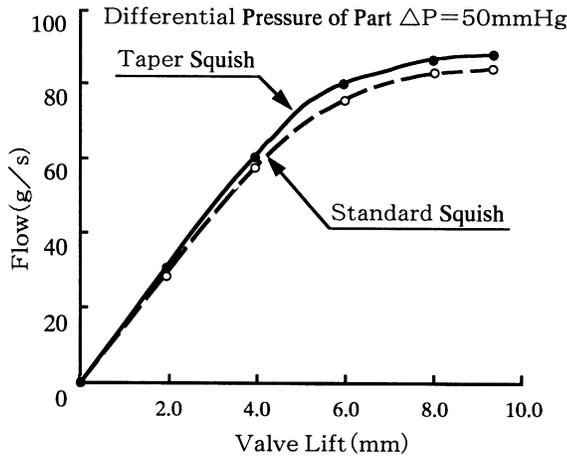
Figure 11. Comparison of Flow Rate Characteristics
