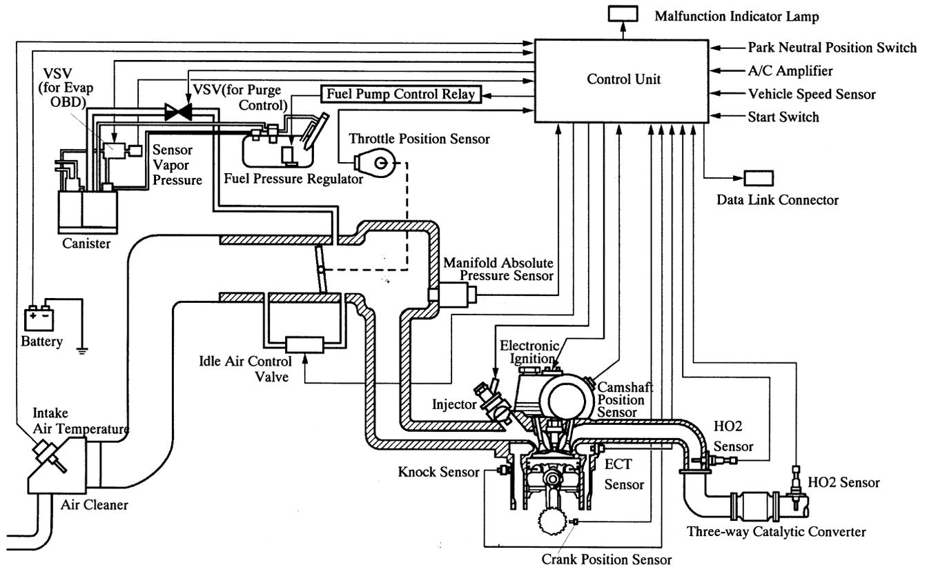
Figure 21. Engine and Emission Control System
