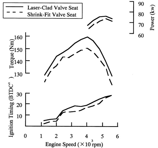
Figure 9. Effect of Laser-Clad Valve Seat
