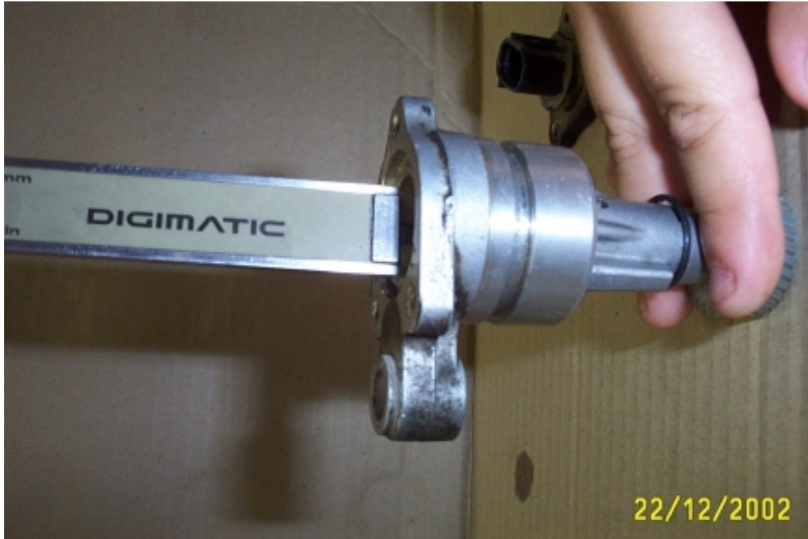
Fig.4 Drive Shaft Depth Std AE101 Shaft & Housing
