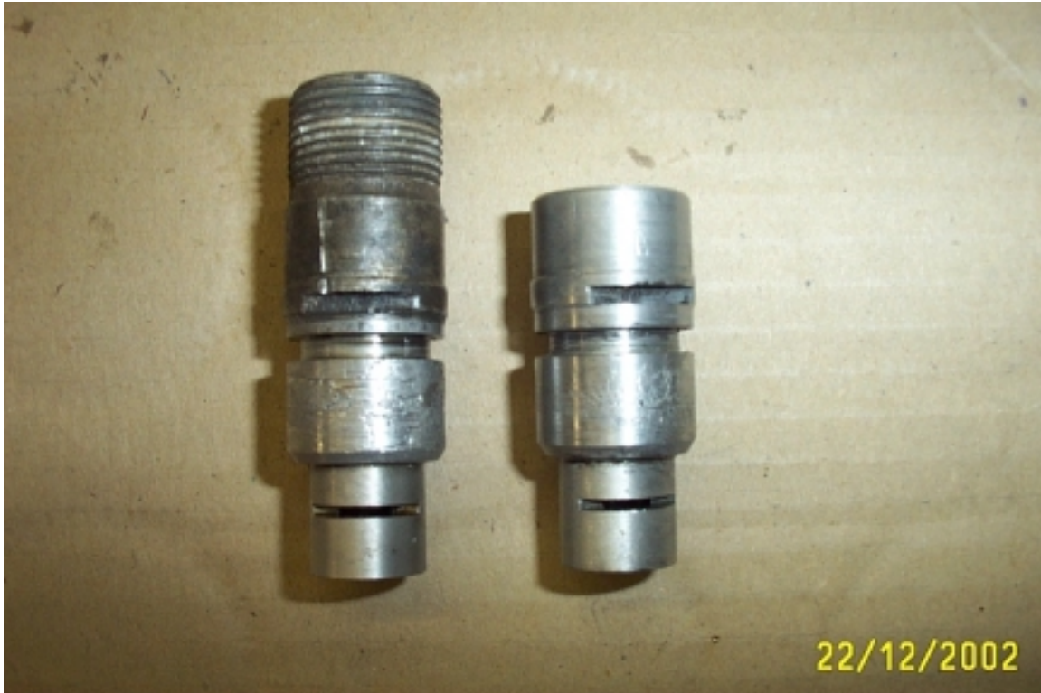
Fig.7 Standard T50 Housing left Shortened Housing right .
