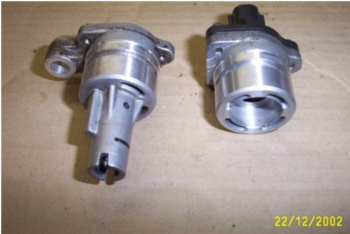
Fig.9 Standard AE101 left Modified right
