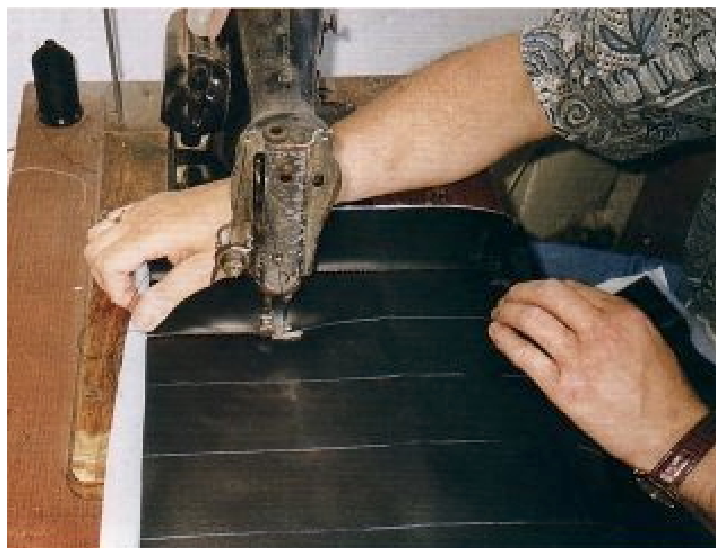
Fig 17.9 The pleats being machine sewn into the "sandwich" made up from the vinyl cover material, foam and calico backing
