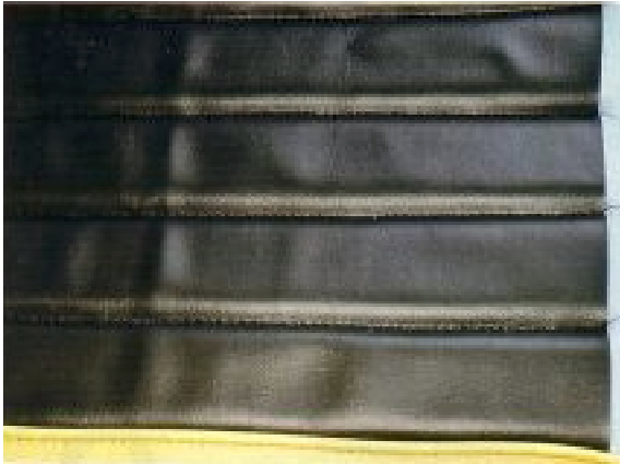
Fig 17.11 Piping sewn to the edge of the panel for the seat bottom
