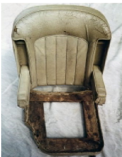
Fig 17.3 A partially stripped oak framed seat from a luxury car
