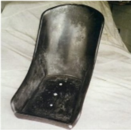
Fig 17.1 Basic racing seat in GRP which can be upholstered
