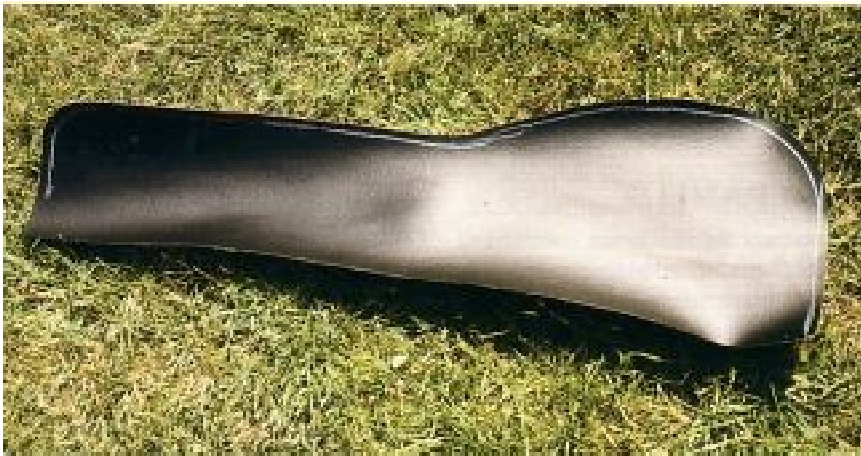
Fig 17.11 Piping sewn to the edge of the panel for the seat bottom
