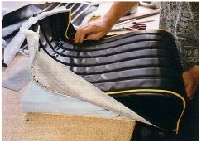
17.13 The completed seat bottom cover is pulled over the foam and the seat base
