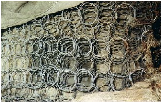
Fig 17.4 Original "innards" of the seat previous seat - springs encased in hessian with horsehair padding
